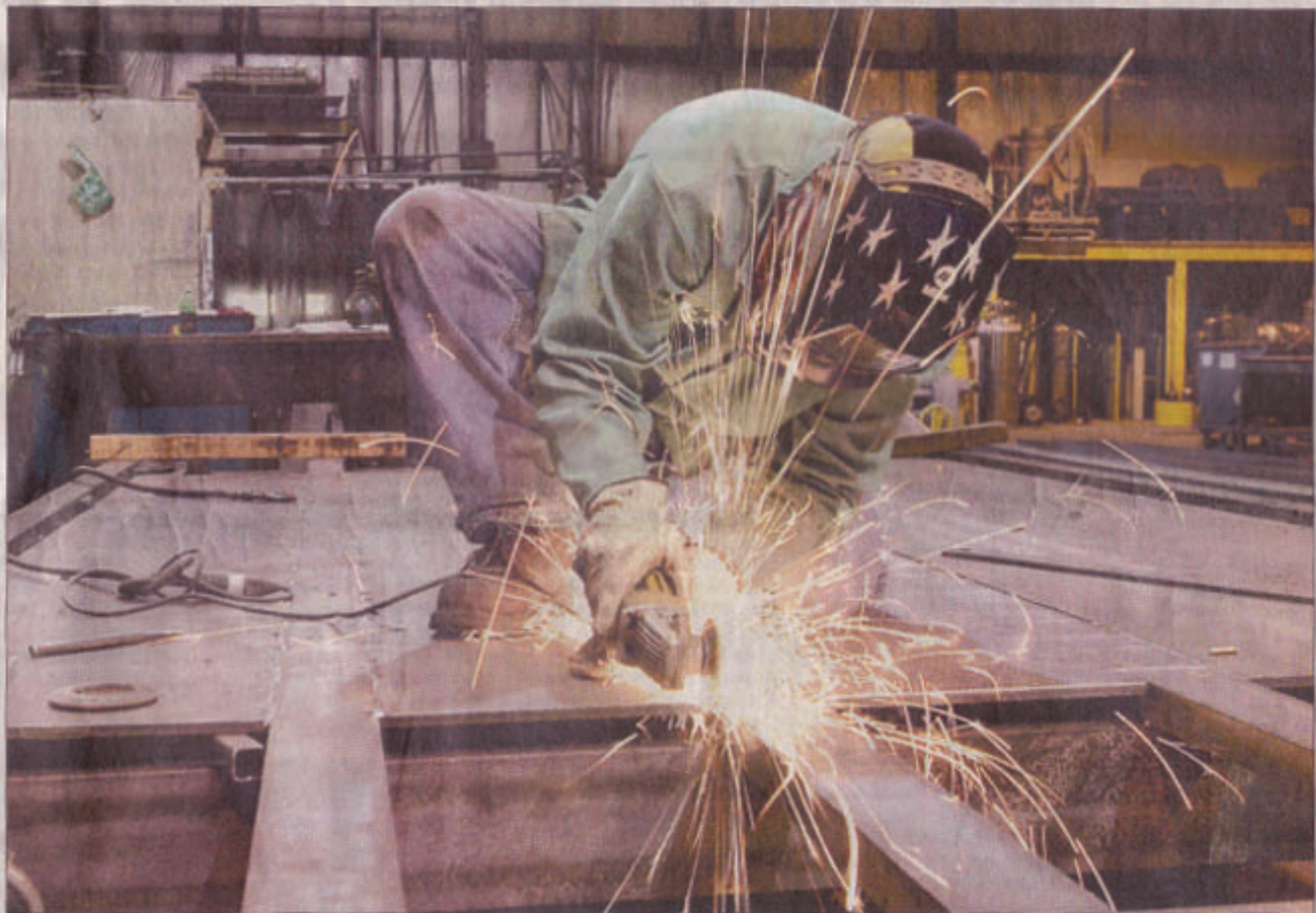
METAL FABRICATOR ERIC CRISCIONE grinds the surface of a steel platform being fabricated at Val-Fab Inc. in Neenah.
